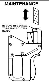
All maintenance or adjustment of the unit requires a metric 5 millimetre Allen Key. An imperial 3/16 inch Allen Key can also be used however it is a poor fit in the screws.
